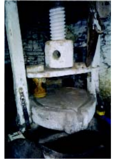
The cider press and its large wooden turning-screw
